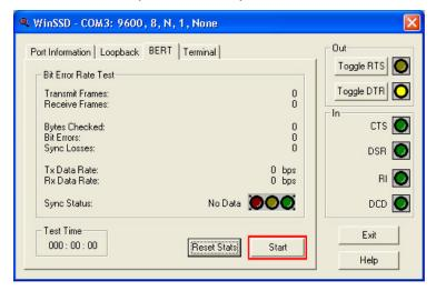
• If the COM port is working properly, the green light will glow and the Transmit Frames and Receive Frames will increase. The Tx and Rx Data Rates will show the calculated data rate. (Pictured below)
