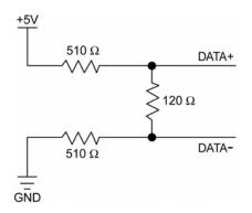
$120\Omega$  termination resistor always present between Data+ and Data-
