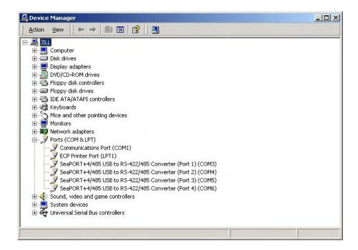
You can access your new COM: ports by using the assigned COM: identifiers as shown above. In this case, it is COM3, 4, 5 and 6. However, this assignment will vary from system to system. At this point, the hardware is recognized and ready to use.
